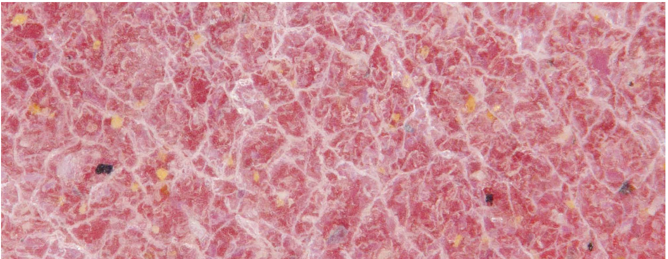
Microscopic view of the grain pattern of the WET&DRYFINISH Foam Abrasive Discs.
