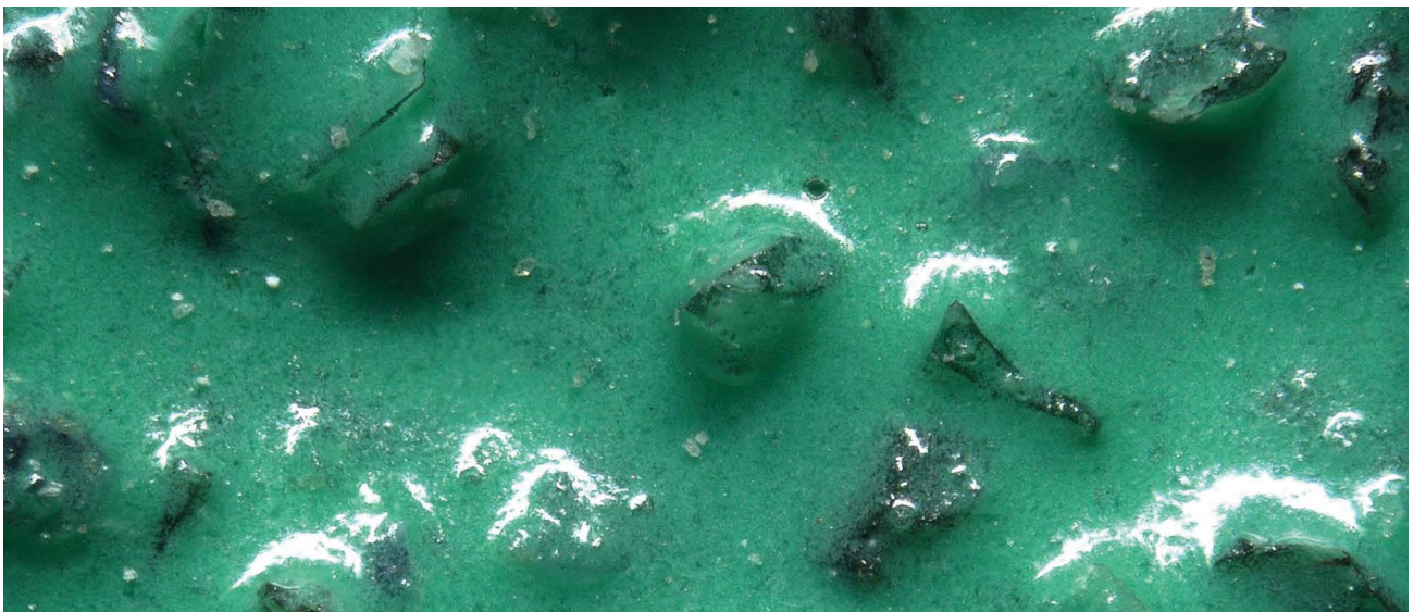
Microscopic view of the grain pattern of the PROCUT Film Abrasive Discs and Sheets.
